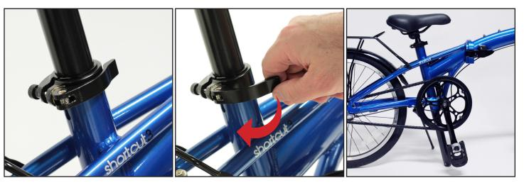
Closed / locked quick-release lever.
