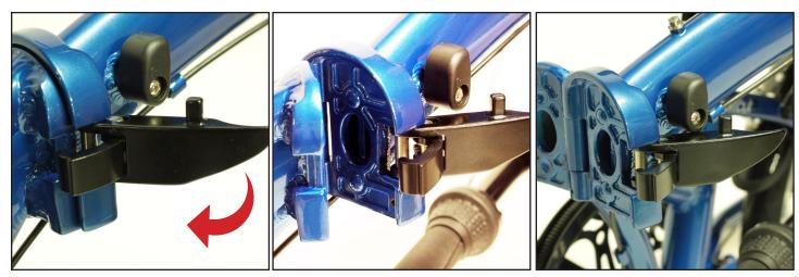
Connector hook will begin to disengage from the frame as you swing the lever open. The connector hook is now disengaged and you can begin folding the frame. Fold the front frame 180 deg. towards the left side of the bike until the front wheel meets the rear wheel.
