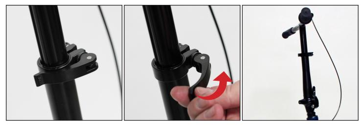
During use the quickrelease should be in the closed / locked position. To adjust handlebar height up or down swing the lever wide open. Do not twist the lever. If handlebar moves while in the closed position add tension to the adjustable nut on the opposite side. Handlebar can now be adjusted up or down. Do not raise above max height line marked on the bar.
