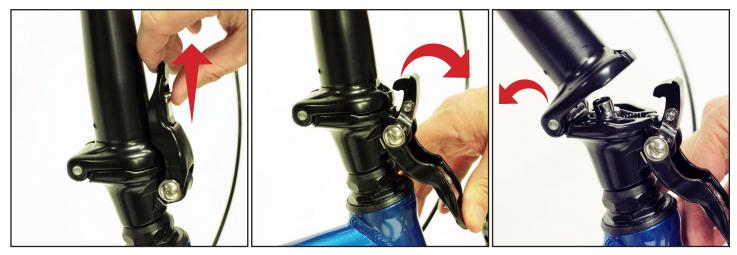
Slide the chrome quickrelease safety lock upward.
